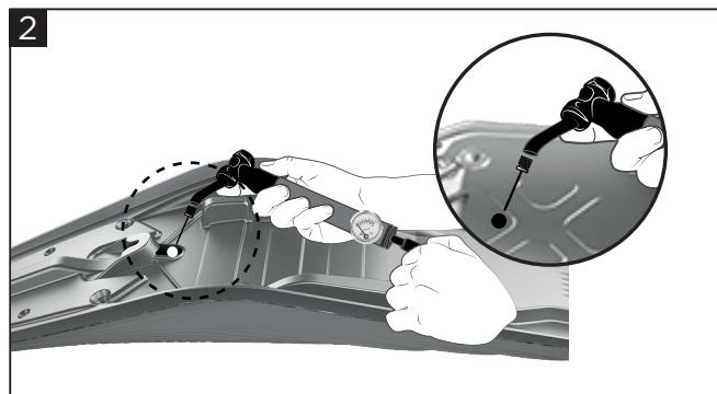
**To inflate the internal bladder connect the included needle tip to the pump and insert into the seat. For best results lube the needle with a silicone based lubricant.**
